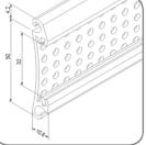
Constructed with high quality aluminium and alloy for strength and durability. Perforated slats permit subtle vision, light and airflow.
